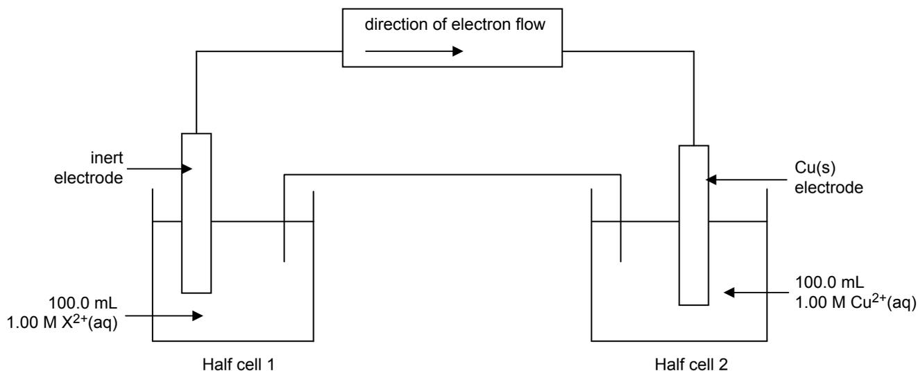
After discharging 2654 C of electricity, the concentration of the  $X^{2+}(aq)$  in solution in half cell 1 was found to be 0.725 M. The volume of the solutions in the two half cells had not changed.
