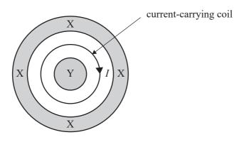
The force, *F*, acting on the current-carrying coil is directed into the page.
