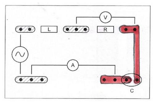
The question was attempted by most students. Students needed to draw in the substantial artwork of the missing copper tracks, but many only responded with fine lines as drawn in the circuit schematic diagram provided. The wiring connections of the AC supply, meters and switch were provided through the provision of pin holes in the PCB where wires could be inserted.
