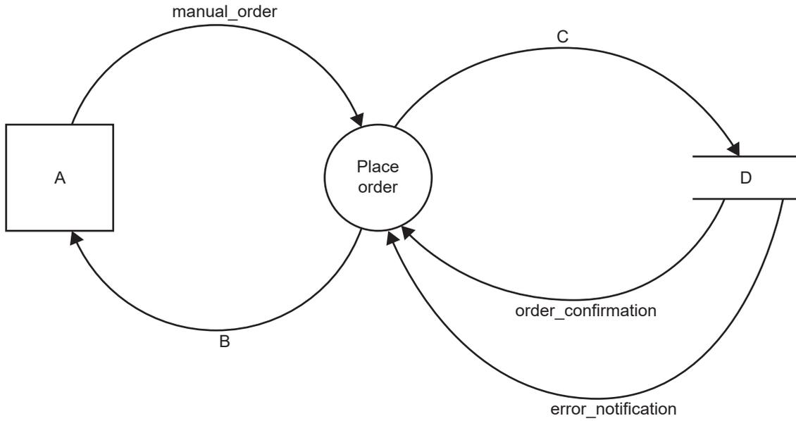
The data flow diagram above shows the ‘Place order’ process for ordering items.
