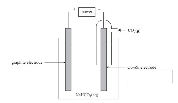
The following half-cell reactions occur in the  $\rm CO_2-H_2O$  electrolysis cell.
