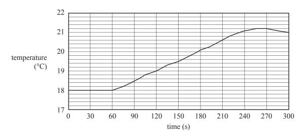
The calorimeter was calibrated using a current of 2.7 A, starting at 60 s. The current was applied for 180 s and the applied voltage was 5.4 V.
