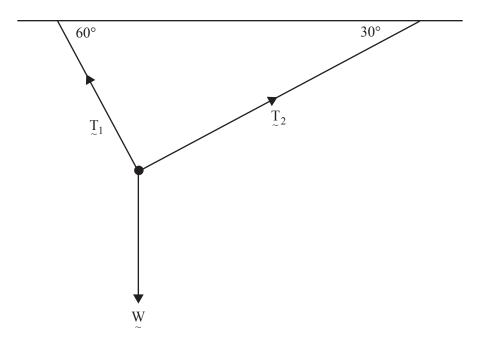
The diagram above shows a mass suspended in equilibrium by two light strings that make angles of 60° and 30° with a ceiling. The tensions in the strings are  $T_1$  and  $T_2$ , and the weight force acting on the mass is W. The correct statement relating the given forces is
