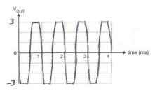
The graph shows clipping at the top and bottom at +3 and -3 volts. The graph is also inverted, the period is the same as the input and it is centred about zero.
