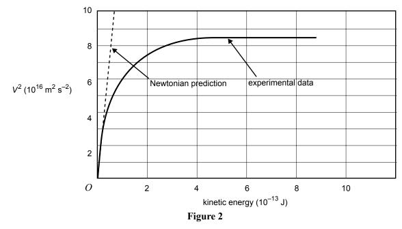
The solid curve in Figure 2 shows the variation of  $v^2$  as a function of KE, as measured in the experiment. The dashed curve is the value of  $v^2$  calculated using the Newtonian expression for kinetic energy.
