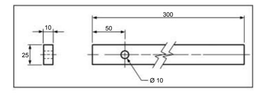
You are required to design a drilling fixture for a production situation that enables the operator to drill the  $\emptyset$  10 mm hole.
