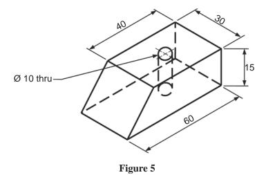
Calculate the volume, in cm<sup>3</sup>, of the wedge shown in Figure 5 above.
