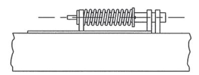
The detailed drawing (Figure 3) shows that the locking pin and the hole in the locking lug are both  $\emptyset$  25. If the **general** tolerance is applied to these two diameters they may not fit together.
