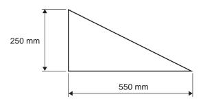
Triangular pieces of metal of length 550 mm and width 250 mm, as shown above, will be guillotined from one sheet of sheet metal measuring  $2.4~\text{m}\times1.2~\text{m}$ .
