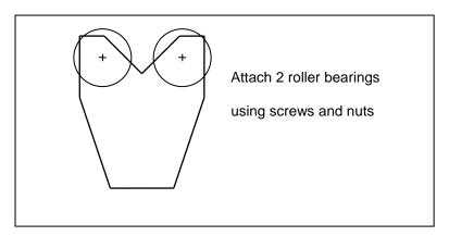
Most students simply rounded off the bottom of the vee on the support bracket, which is not suitable for eliminating wear.
