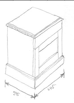
Students were required to complete a perspective sketch of the bedside cabinet. Marks were allocated for creating a perspective sketch, sketching the correct item, including all visible parts, showing details of grain and mouldings, including overall dimensions.
